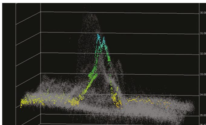
Figure 2. RAMMS point cloud (grey) vs. SHOALS on target feature
