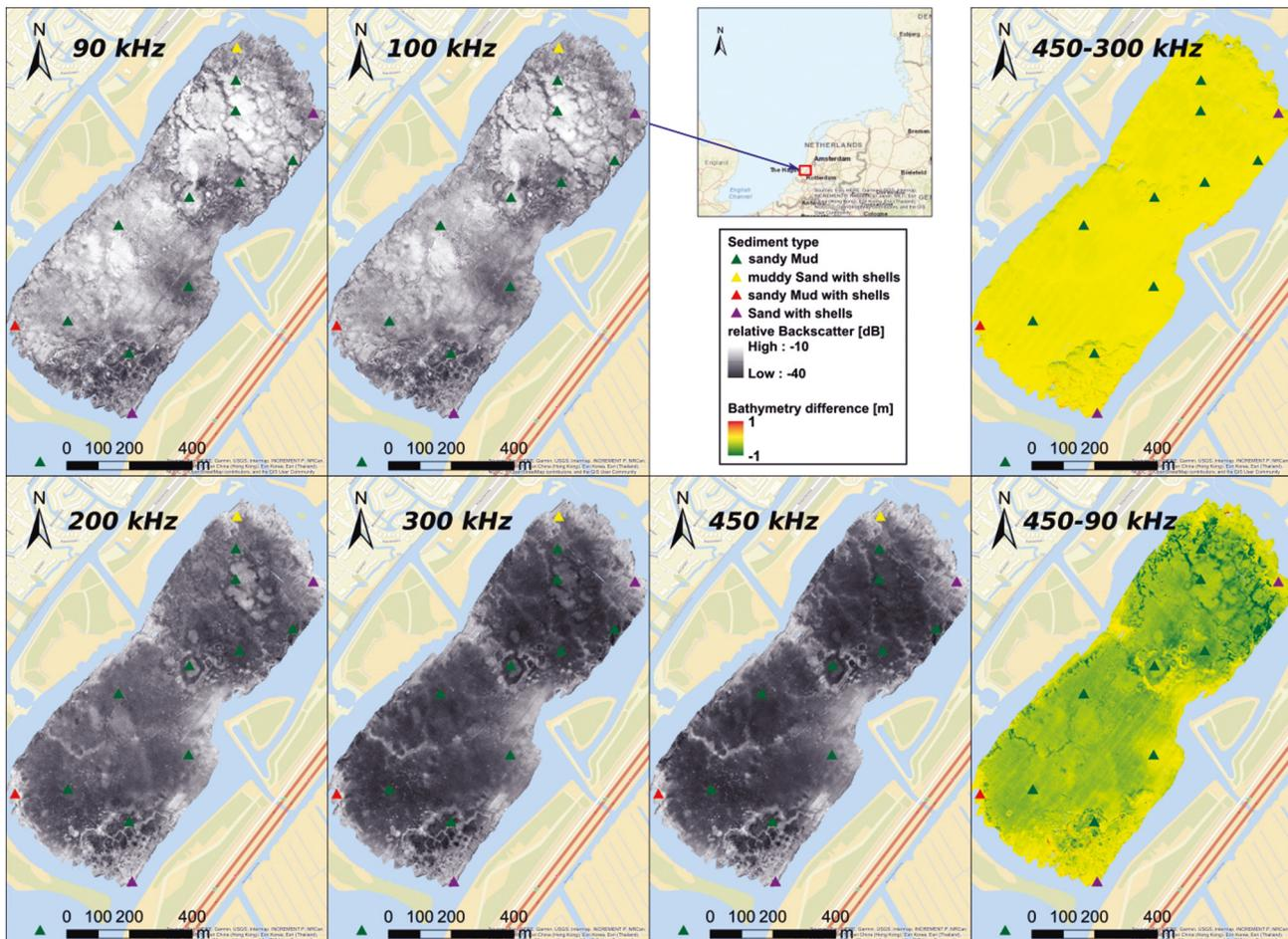
Figure 1. Multi-frequency backscatter maps (90, 100, 200, 300, 450 kHz) and bathymetry difference maps (450–90 kHz and 450–300 kHz) from the Vlietland Lake, The Netherlands. The spatial resolution is 1 m by 1m
