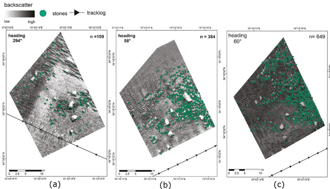
**Figure 1. Sonographies of the study area displayed in three different levels of resolution. Green dots symbolize detected stones. (a) resolution: 0.1m/pixel, (b) resolution: 0.05m/pixel, (c) resolution: 0.01m/pixel**
