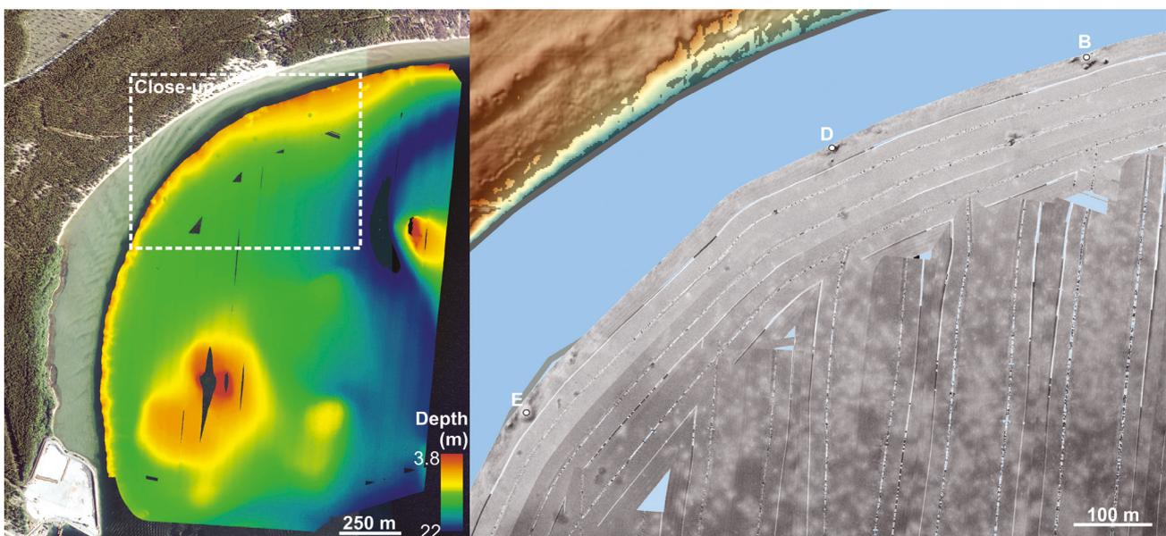
Figure 1. Multibeam bathymetric image (left) and a sidescan sonar close-up image (right) of pockmarks at the Hanko submarine groundwater discharge site
