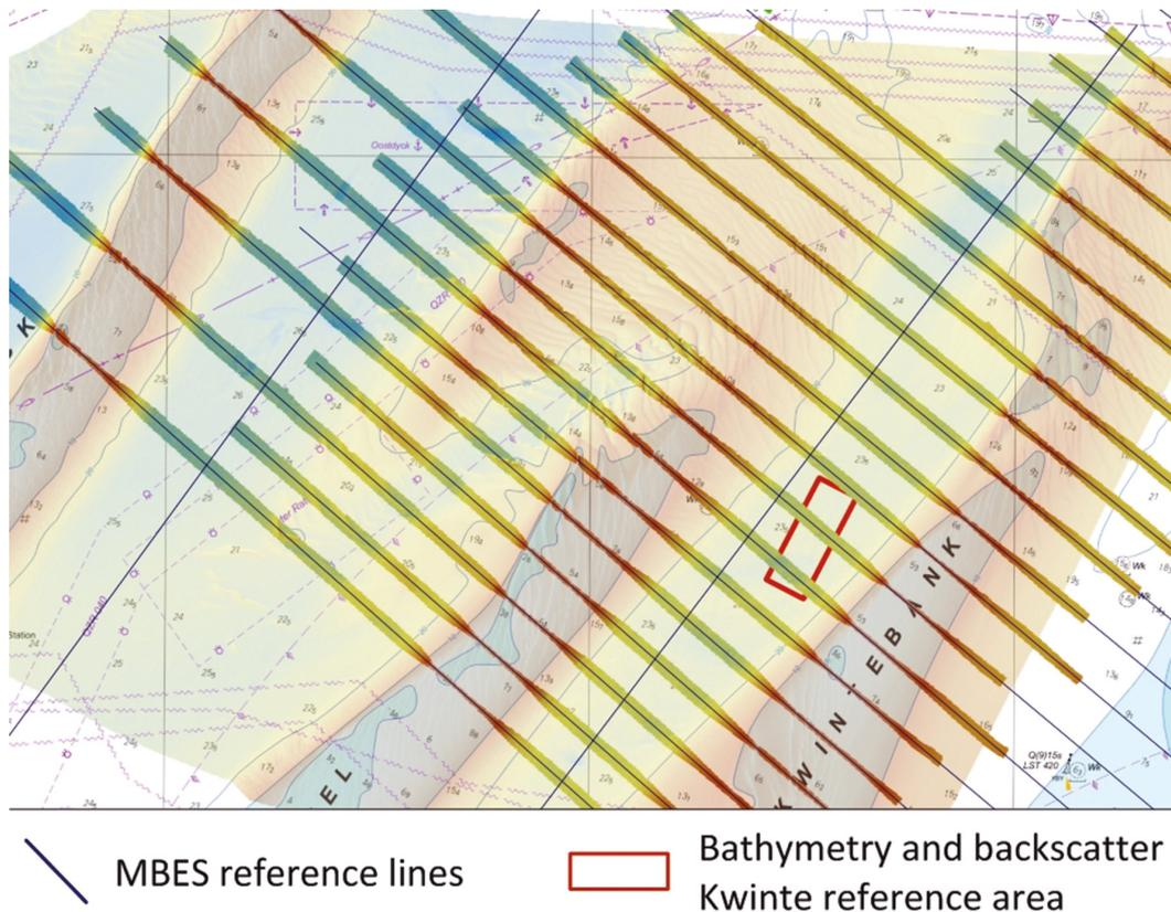
**Figure 2.** Part of Flemish Banks area (black rectangle in Fig. 1). MBES reference lines are surveyed each year. The Kwinte reference area is used to control the bathymetry and the backscatter accuracy and stability. Background: Hydrographic chart 102 “Frans-Belgische Kust van Duinkerke to Oostende” Vlaamse Hydrographie December 2018; Reference DTM of sand extraction Zone 2 FPS Economy; Survey 1608 RV Belgica EM3002d 22–23/02/2016
