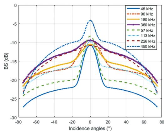
**Figure 1. Fitted model of the calibrated EK80 angular backscatter measurements for the “Rascass” area at different frequencies**
